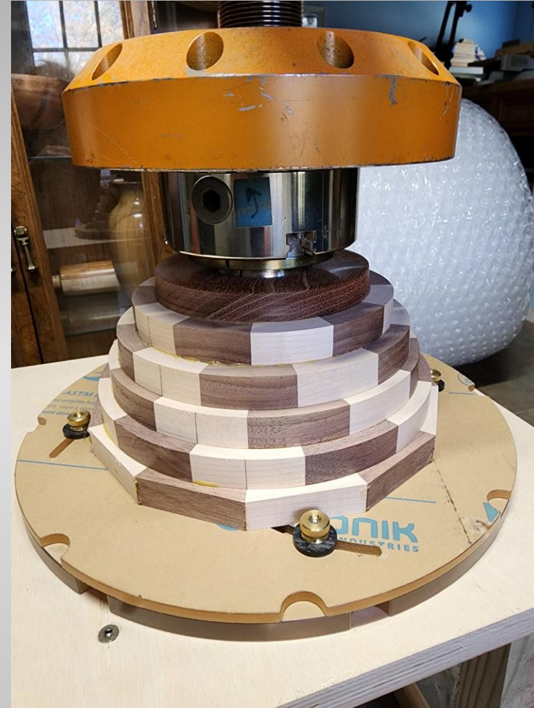
Approximately 25 pounds of weight used for clamping pressure
