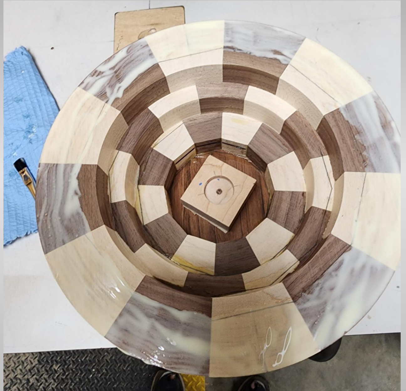
Glue applied for stacking the next ring
