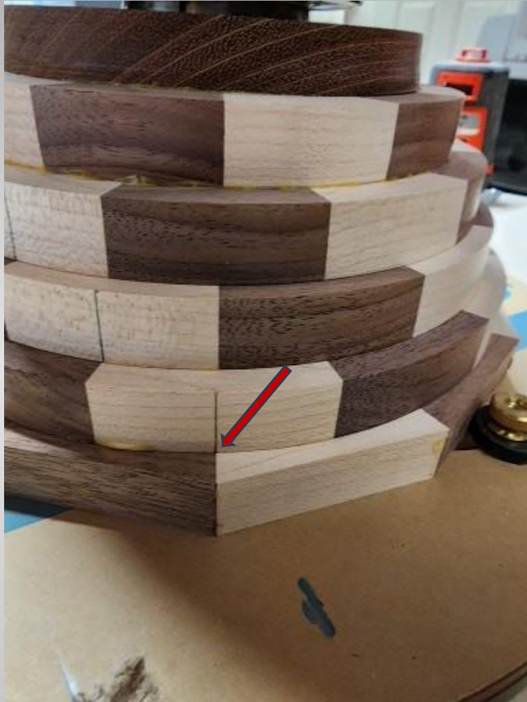
Center of maple segment aligned with bottom ring glue line
