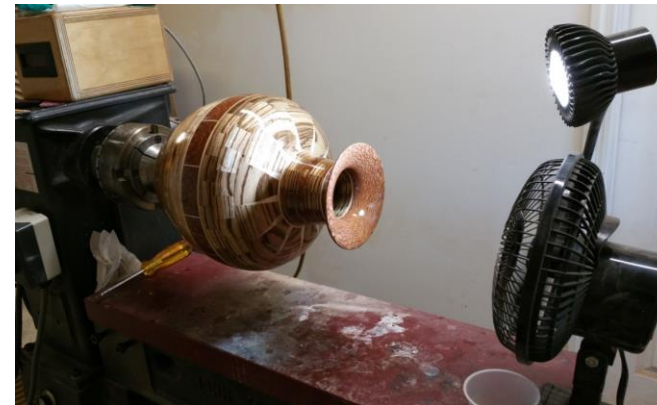
A small fan speeds up the flashing over point for the inside of bowls and vases
