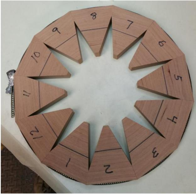
Segments glued and clamped with a hose clamp. Be sure to remove all glue squeeze out from points to allow triangles to fit all the way in.
